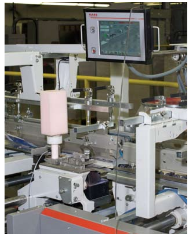
The Valco Cincinnati OT-120 touchscreen data entry terminal aboard the EXPERTFOLD folder-gluer from Bobst is utilized to ensure 100-percent gluing and finishing quality assurance.
